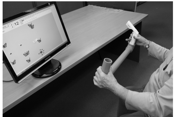
Figure 2: Cywee game controller fitted to bilateral handlebar.
